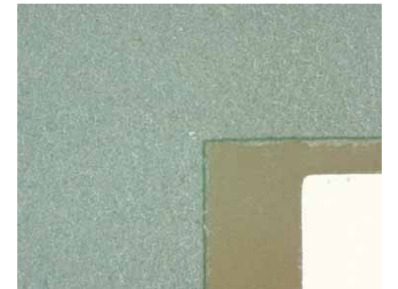
Corner crack: Thermal Cycle -40°C(30min.)⇔140°C(30min.) Above 500cycles
